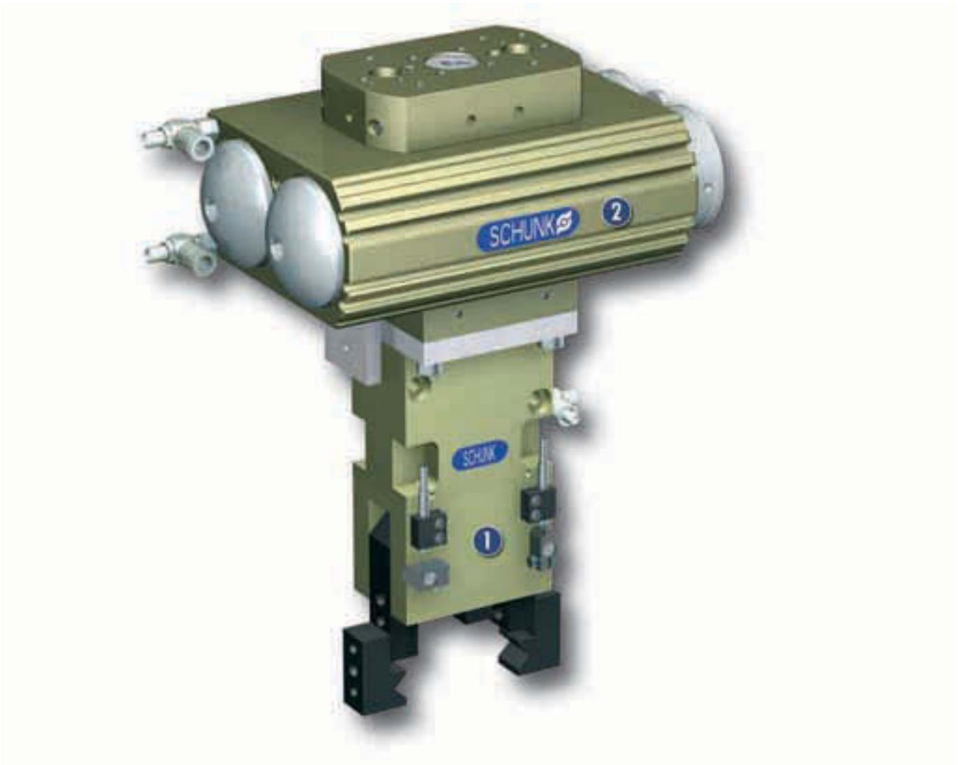
Rotating/gripping combination for handling small wheel spindles. The 180° opening angle of the gripper eliminates the linear unit that would otherwise be necessary.
